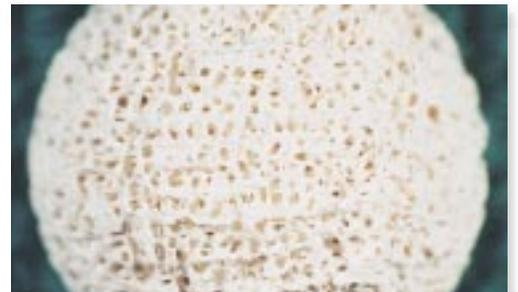
The Bio-Eye implant is made of hydroxyapatite.
